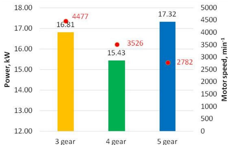
Fig. 4. Power and motor rotation frequency at  $90 \text{ km}\cdot\text{h}^{-1}$
