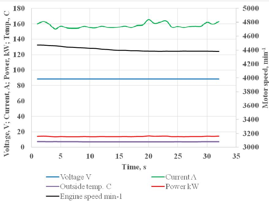
Fig. 2. Results of road tests performed in third gear at 90 km·h<sup>-1</sup>
