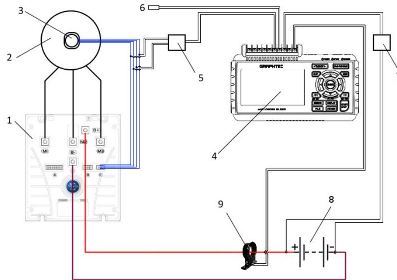
Fig.1. **Scheme for connecting experimental equipment:** 1 – motor controller; 2 – electromotor; 3 – electromotor speed sensor; 4 – data logger; 5 – frequency-voltage converter; 6 – temperature sensor.; 7 – voltage divider; 8 – 96 V accumulator; 9 – current sensor
