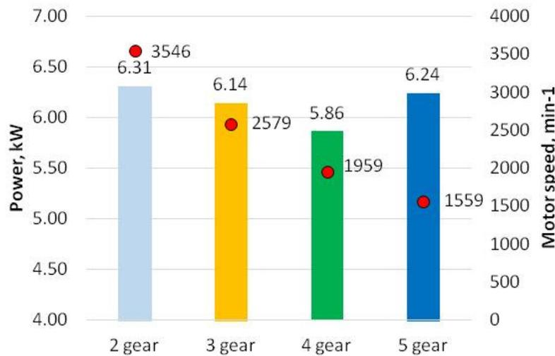
Fig. 3. Power and motor rotation frequency at 50 km·h<sup>-1</sup>
