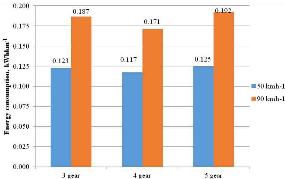
Fig. 5. Energy consumption at 50 km·h<sup>-1</sup> and 90 km·h<sup>-1</sup>
